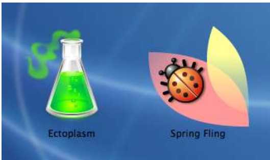
The Power of "Deep" 8-Bit Masks (fig. 1) - If you look closely at these two icons, you can see how the background pattern of the desktop shows through the translucent areas. This is accomplished by setting different opacity levels in Photoshop layers and using them as the icon's mask data. Experimenting with these methods can create some exciting effects on the desktop.
